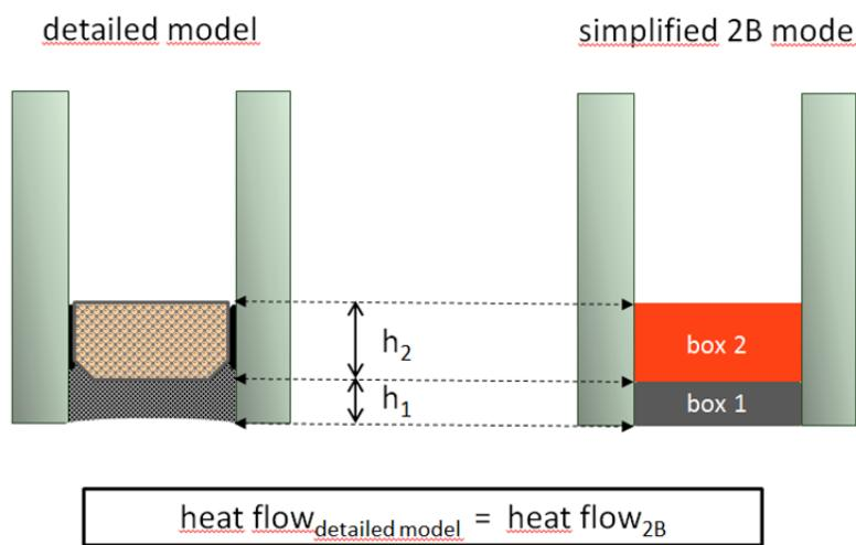
To compare the thermal performance of glass edge bond, usually a full thermal simulation according to EN 10077-2 including window frame and glass is required, which produces comparable  $\Psi$ -values of spacers, if simulated under exactly the same frame conditions.
