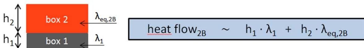
The two-dimensional heat flow through a box of a fixed width (cavity) at a defined temperature difference  $\Delta T$  is proportional to the height of the box and to the thermal conductivity value, i.e. it is proportional to the product  $h \cdot \lambda$ .
